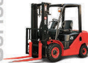
LPG / Gasoline / Diesel Counterbalance 1 to 3.5 tonnes
