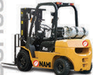
LPG / Gasoline Counterbalance 1 to 7 tonnes
